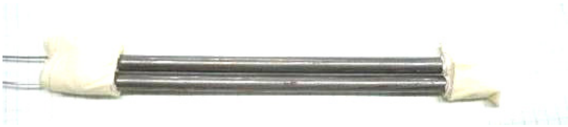
Figure 22. Electrochemical Probe Before Grouting
