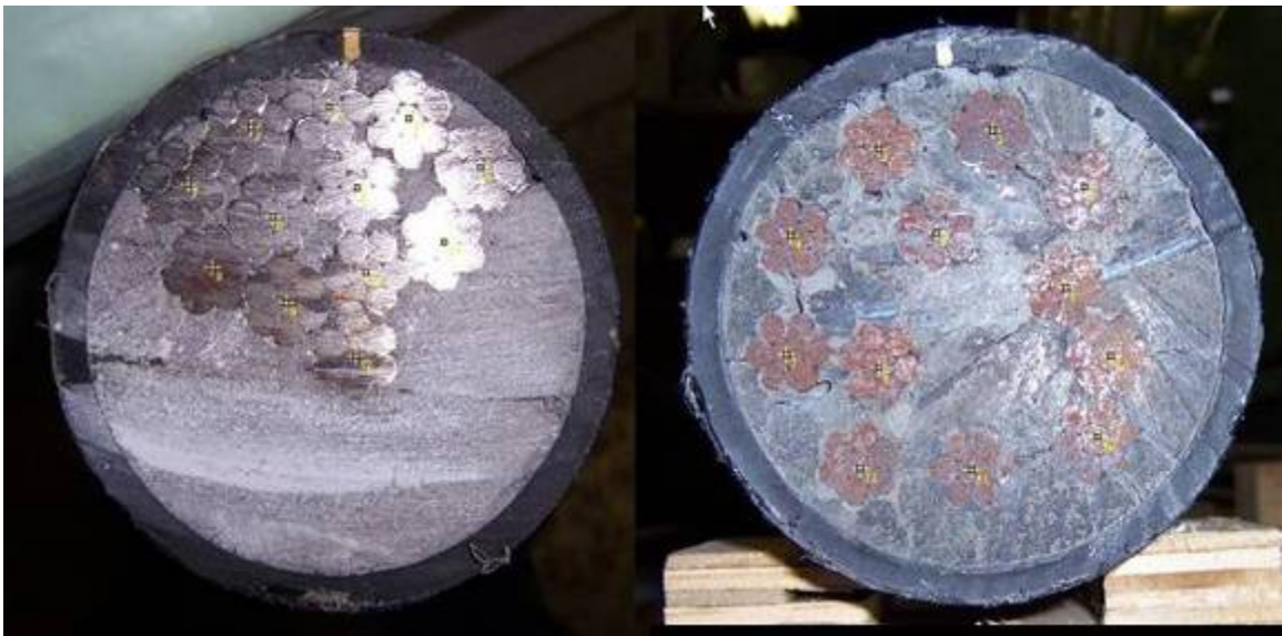
Figure 9. Strands Configuration; Tendon 13A, Horizontal Section [10]
