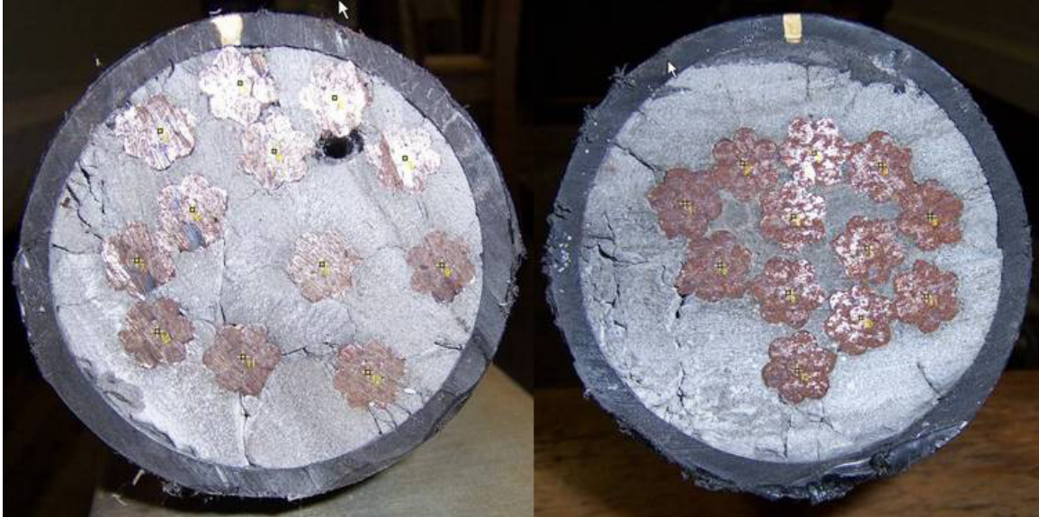
Figure 8. Strands Configuration, Tendon 13A Sloping Section [10]
